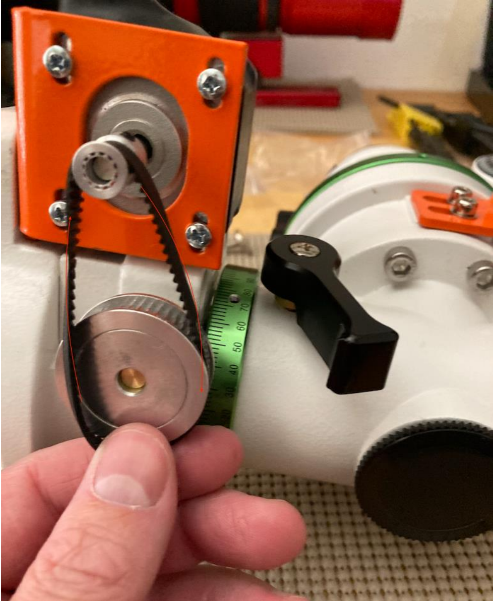
Install the belt and put it on the small pinion (the motor gear) and slowly turn it around the main gear
